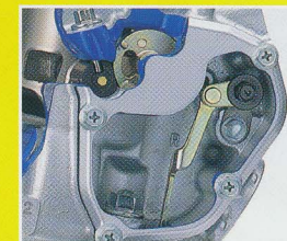
New exhaust valve control system
