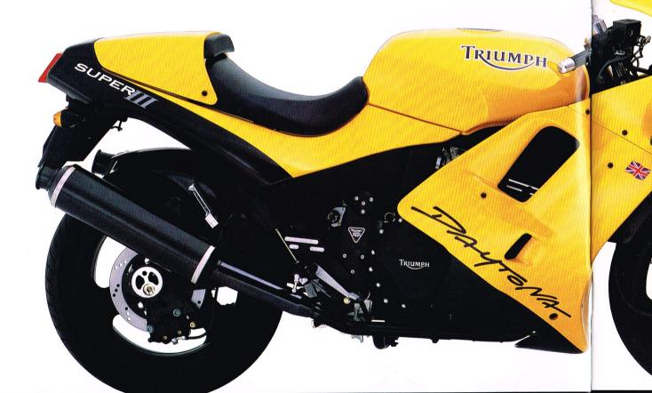
**Engine and Transmission.** Based on the standard specification Daytona 900 - liquid cooled, 3 cylinder, 885cc DOHC engine with a bore and stroke of 76 x 65mm, the
