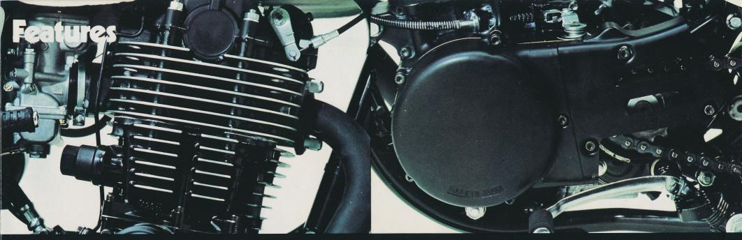
**Overhead cam, four-stroke single,** develops smooth power over a broad range. Typical of big bore singles, there is quick response and abundant torque even at low rpm's.
