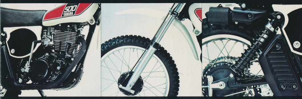
**Single-downtube cradle frame** is light but strong. The low profile creates a low center of gravity for better balance and positive handling.
