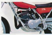
In order to assure that the TY175C will be able to withstand the severe treatment encountered on the roughest section, the frame design is a doublecradle type. This frame, with its hightensile-strength, tubular-steel construction, is based on the frames of the famous YAMAHA Motocross and Road Racer machines which have been consistent championship winners on leading
