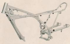
The TY250B utilizes an extra-durable diamond-type desing. This frame design features a more slender tube, through the use of high-tensile-strength steel, to attain a lighter frame without sacrificing any of the machine's ability to withstand severe punishment. Also, the geometrical form of the diamond frame is ideally suited to withstand large stresses and strains encountered from any direction while maintaining overall machine stability.
