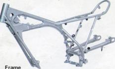
The TY250C utilizes an extra-durable diamond-type design. This frame design features a more slender tube, through the use of high-tensile-strength steel, to attain a lighter frame without sacrificing any of the machine's ability to withstand severe punishment. Also, the geometrical form of the diamond frame is ideally suited to withstand large stresses and strains encountered from any direction while maintaining overall machine stability.
