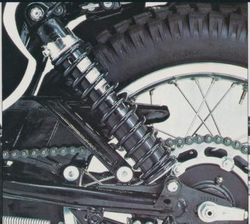
Forward-mounted nitrogen/fluid shocks provide greater rear wheel travel for better control, consistent traction and superior, fade-resistant dampening.
