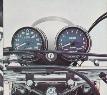
Enduro instrumentation includes speedometer, tachometer and re-settable trip meter. Sealed-beam headlight provides bright automotive type illumina-
