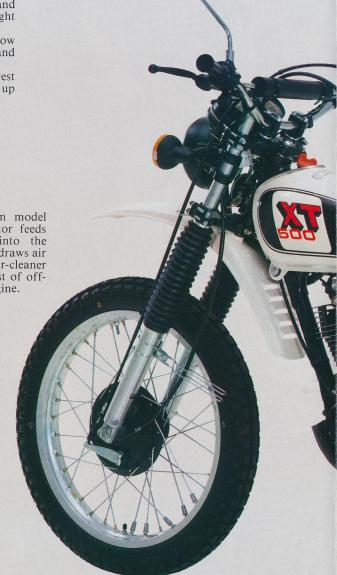
Ignition and batterycharging are handled by a flywheel magneto. The extra weight of the magneto flywheel on the crankshaft is also a great added advantage to the already-strong, lowspeed pulling power of the XT500.
