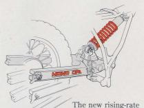
Monocross suspension system features a box-section alloy swinging arm pivoting on needle roller bearings. Its movement is controlled by a system of lightweight linkage arms and a single gas/oil shock absorber with adjustable spring pre-load and rebound damping. Monocross provides 235mm of rear wheel movement plus a lower centre of gravity and a centralized weight mass.
