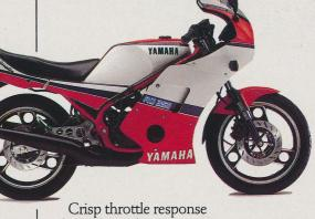
Crisp throttle response throughout the rev range is assured, by the unique YPVS system, which matches exhaust port timing to engine speed, giving one of the widest spreads of power, of any two-stroke, and the smoothest possible mid-range running. So successful is this engine, that it's powering machines, in only a slightly re-tuned state, to victory in Formula II races!
