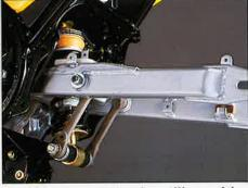
The Monocross suspension utilizes a rising rate linkage acting on a single gas/oil shock mounted low behind the engine for optimum weight placement. It provides supple wheel travel over small bumps, while assuring precise control for hard riding.
