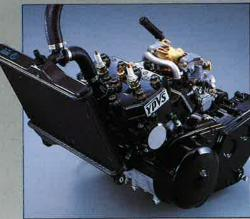
The liquid cooled, 347cc, two-stroke twin features the patented Yamaha Power Valve System (YPVS). It consists of exhaust port valves that give variable porting, operated by a servo motor that is controlled by a microprocessor to coincide with engine requirements and rider demands. The result is substantial torque in the low- and midranges, with phenomenal power on the upper end.
